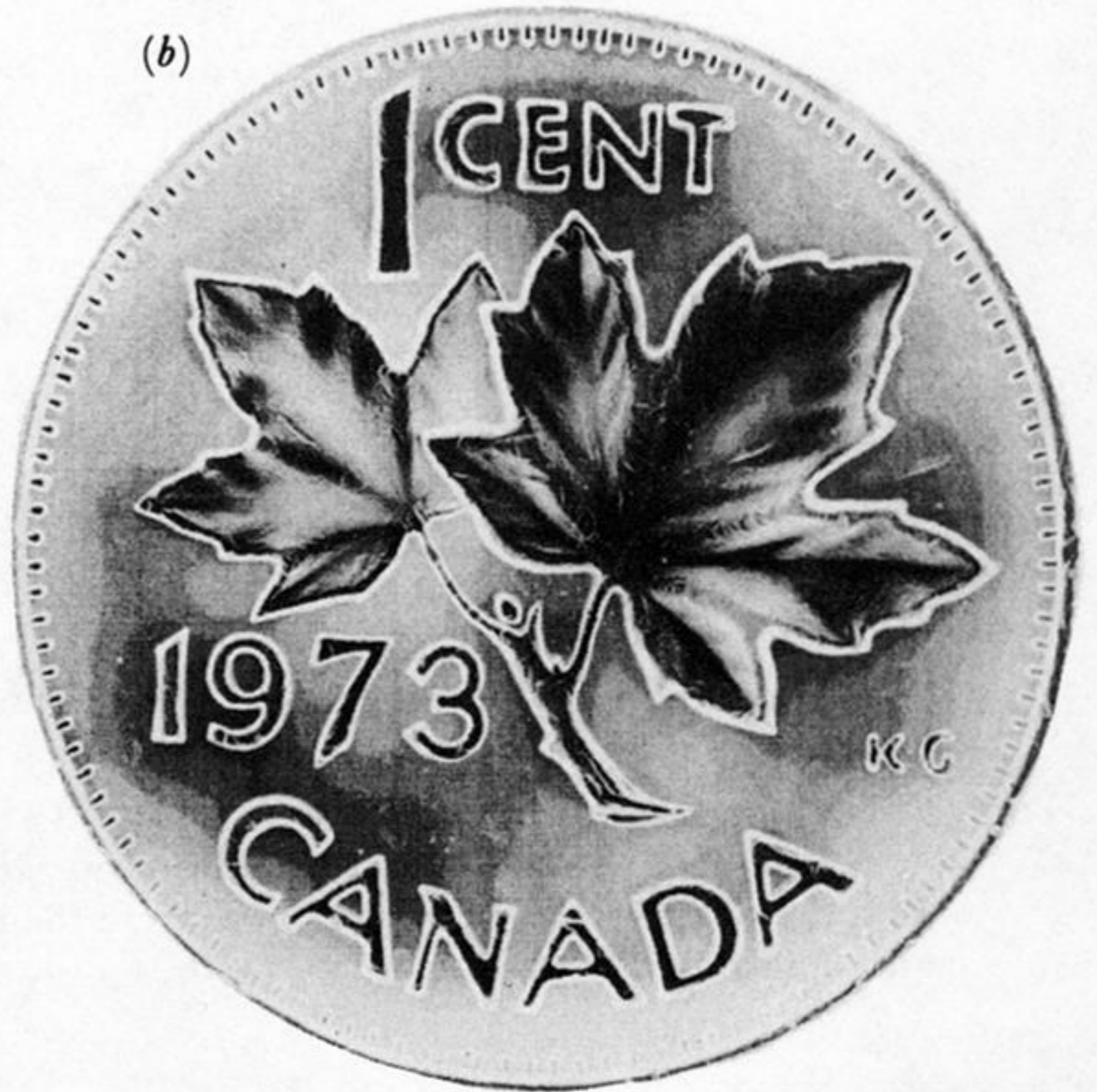
FIGURE 17. (a) Direct reflection image from obverse surface of Canadian penny; same 50 MHz transducer as figure 14, d_{sc} = 0.025 mm. (b) Reverse face of coin. The penny is 19 mm in diameter.
