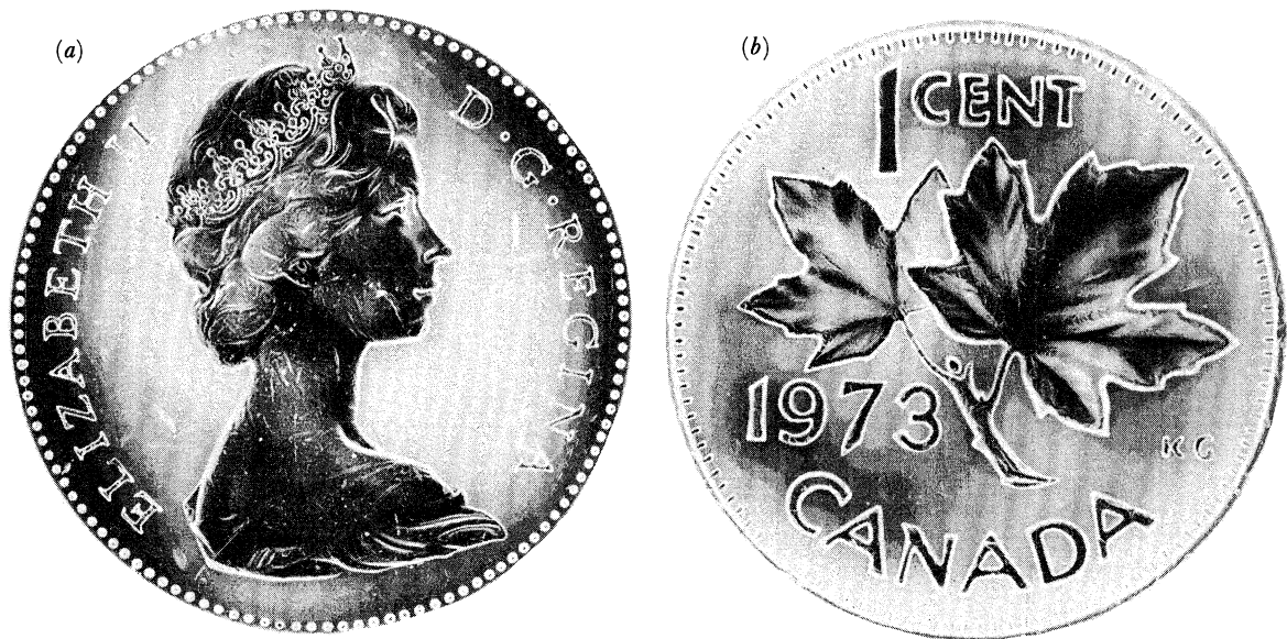
FIGURE 17. (a) Direct reflection image from obverse surface of Canadian penny; same 50 MHz transducer as figure 14, d_{sc} = 0.025 mm. (b) Reverse face of coin. The penny is 19 mm in diameter.
