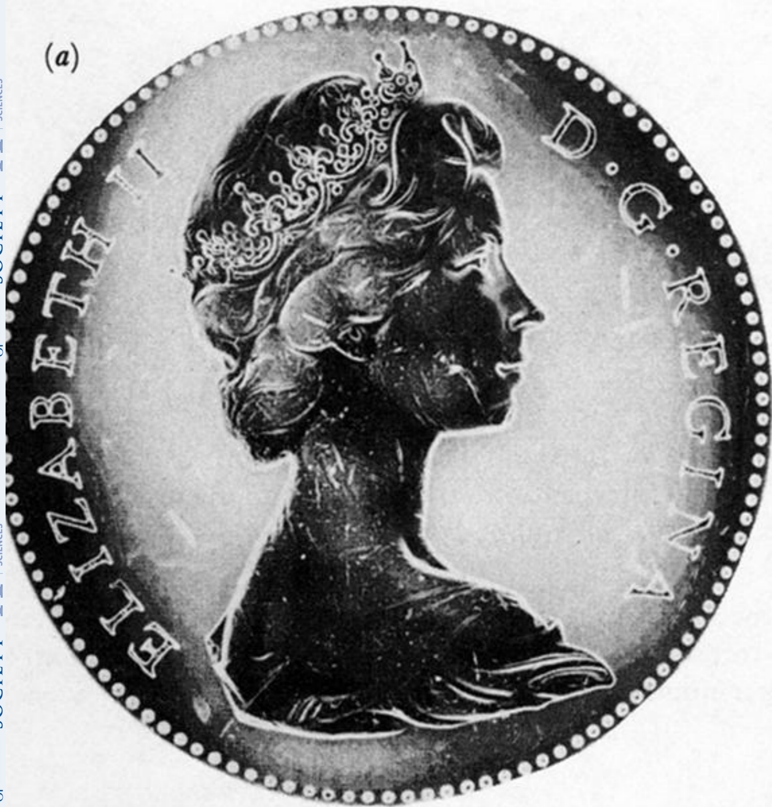
FIGURE 17. (a) Direct reflection image from obverse surface of Canadian penny; same 50 MHz transducer as figure 14, d_{sc} = 0.025 mm. (b) Reverse face of coin. The penny is 19 mm in diameter.
